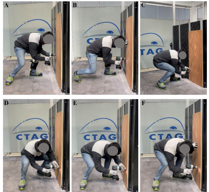
Fig. 3. Snapshots of the use case performed at a simulated industrial scenario ((A)–(C), top) wearing and ((D)–(F), bottom) not wearing the exoskeleton prototype.
