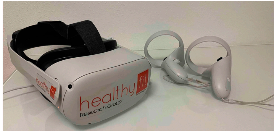
Figure 1. IVR Meta Quest II device used in the study; HMD with elite strap and controllers.
