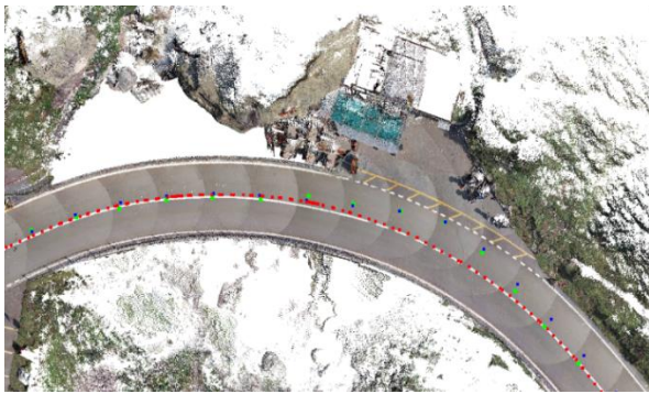
Figure 15. Comparison between the polylines of the ground truth, the alignment and the trajectory close to a car lay-by. Ground truth in red, alignment in green and trajectory in blue.
