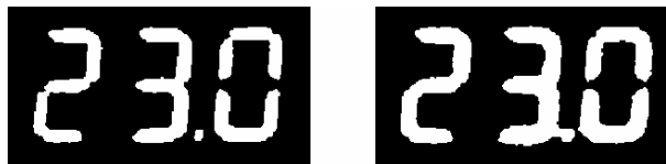
Fig. 7. Left: Peak detection method. Right: iterative Otsu method.
