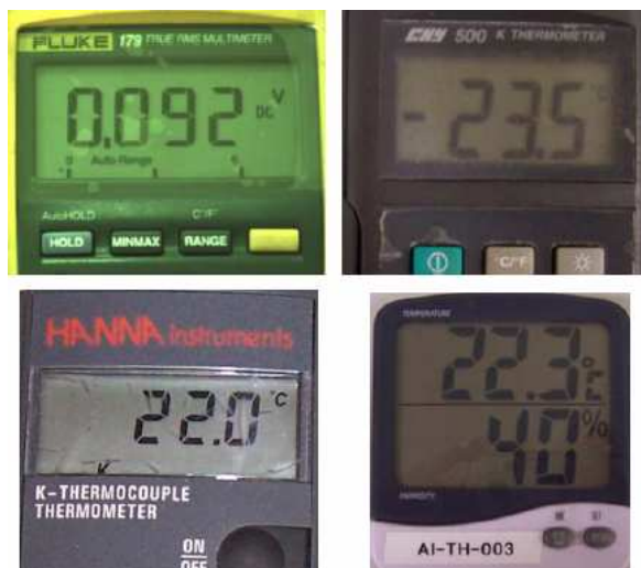
Fig. 1. Examples of different instruments, some of them are showing display defects (bubbles in the first one, stripes in the third one).
