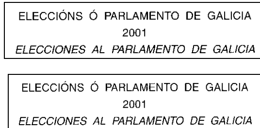
Fig. 10. Binarized portions (above: Otsu, below: Peak Detection)
