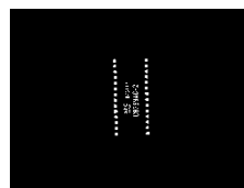
Fig. 2. Otsu method gives a threshold to segment brighter objects
